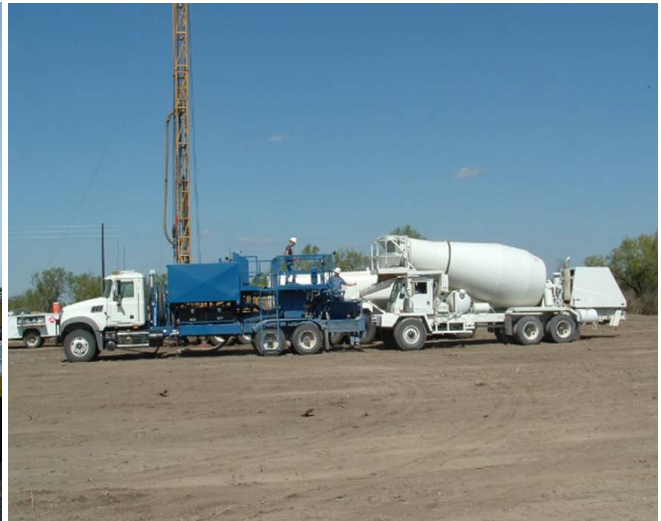
Figure 6: Water well rig used to drill and set 250' surface casing. Figure 7: Cementing equipment for surface casing.
