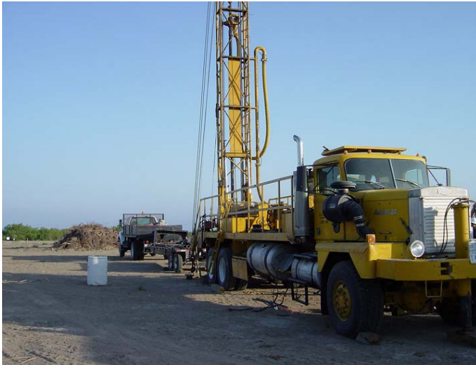
Figure 6: Water well rig used to drill and set 250' surface casing. Figure 7: Cementing equipment for surface casing.
