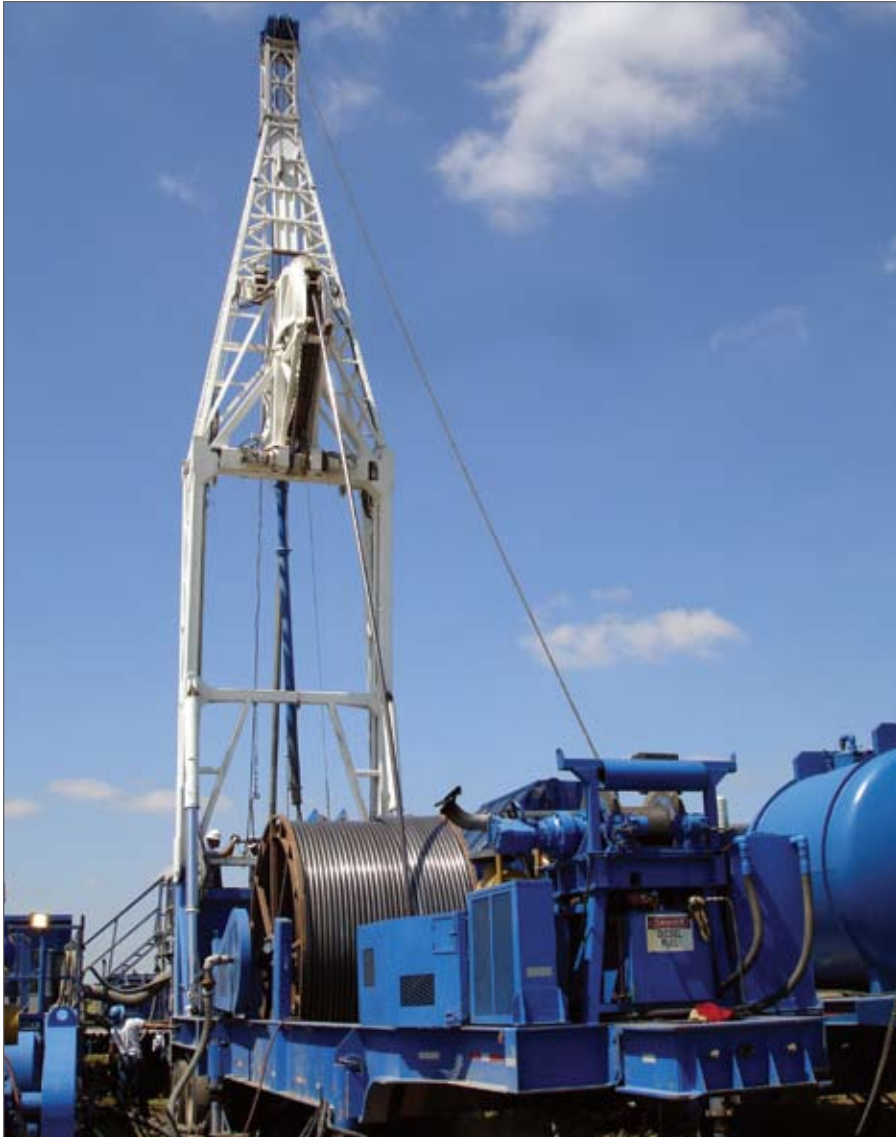
Advanced Drilling Technologies has two CT rigs, each with a 2 7/8-in. coil, that have drilled more than 1,000 vertical wells at no more than 3,900 ft since 2005.
