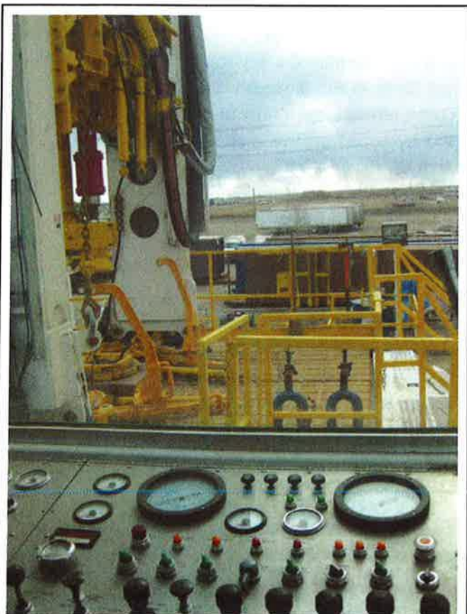
By moving from hydraulic to electric controls, rig manufacturers have made operating coiled tubing rigs more precise and convenient.
